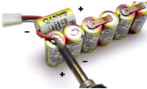
**Caution:** When building battery packs, make sure that positive terminals are always connected to negative terminals on the cells (series connection). Reversing polarity will permanently damage the cells. Solder the positive terminal of the sixth cell to the negative terminal of the seventh cell.
