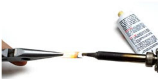
The flux allows the solder to spread very rapidly. This reduces the amount of time spent holding the iron to the cell.
