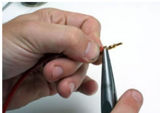
Tin the ends of the wires with the soldering iron and install the bullet plugs onto the end of each wire.
