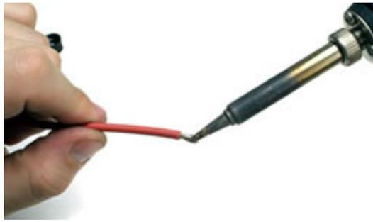
The less heat that you have to apply to your cells when joining the battery bars and wires, the better off your cells will be. Holding a soldering iron onto a battery cell for too long can permanently damage the cell. It's highly recommended to use flux and tin the components first, before assembly.
