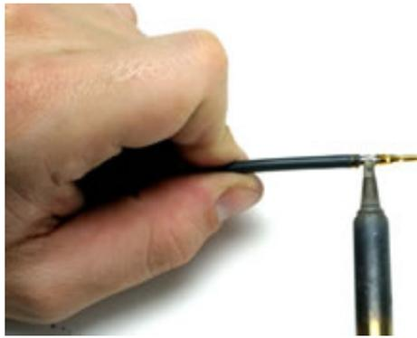
Solder the wires to the bullet plug after crimping them into position. This will keep the wires from pulling out of the plug when unplugging your packs from the ESC.
