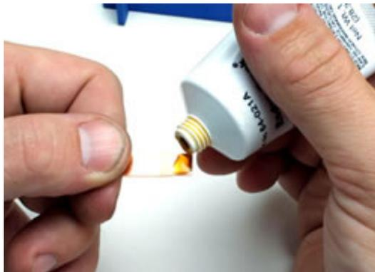
Tinning the ends of the battery bars and also the ends of the wires will also make quick work out of assembling the packs.
