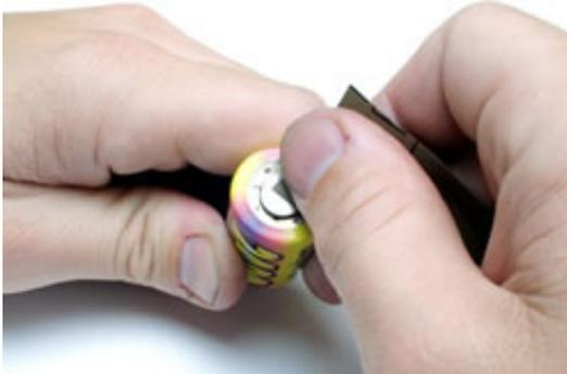
**Step one** – To achieve the best bond possible between the solder and the battery take a small piece of 400 grit sandpaper and scuff the positive and the negative terminals on each battery cell. After cleaning the terminals with some denatured alcohol go ahead and turn on your iron so that it'll be ready. Now place six cells in the battery jig, starting with the 1st cell negative side up. Make sure that the cells line up in a negative / positive / negative sequence.
