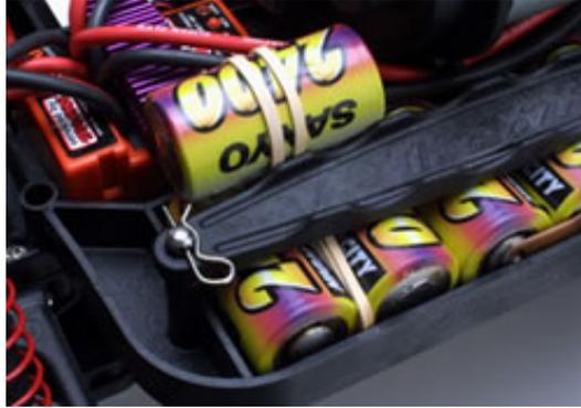
**Tip:** (Wrap the seventh cell with a rubber band first. Then, while holding the cell steady wrap another rubber band around the length of the pack so that it keeps the seventh cell in place.)
