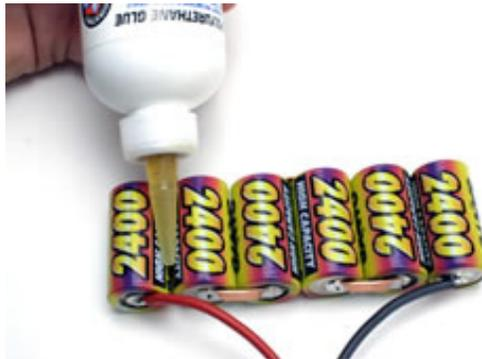
**Tip:** Be sure when applying the glue that you use no more than necessary. The glues mentioned before may take a little while to cure but are very strong. It's very important to use the glue sparingly. Excess glue can get all over the place and can bond things together that you do not want bonded together. Just a small amount of glue between each cell will be plenty.
