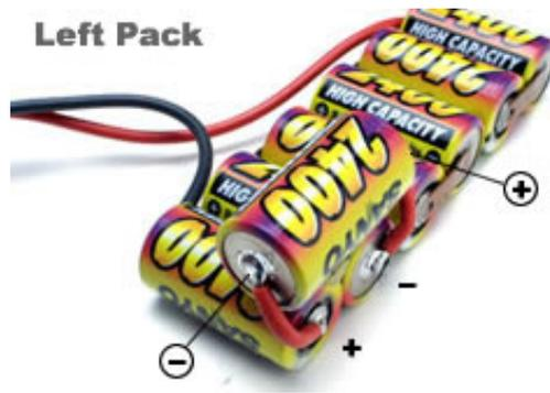
On pack # 1 the seventh is located just above the open terminals and will use the 1 ½" wires to be connected.
