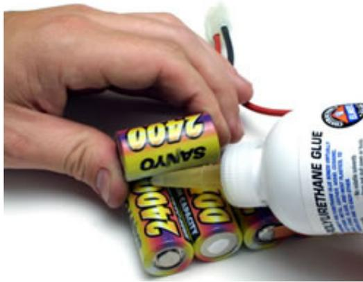
Build the packs so that the seventh cell is towards the rear of the truck and mounted inboard of the chassis to keep them out of danger during a roll over or a crash. The seventh cell is positioned on the side of the pack to clear the battery hold-downs.
