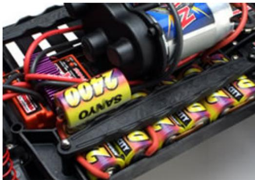
Place the seventh cell across the top and on the side of the last two cells that didn't require a battery bar.
