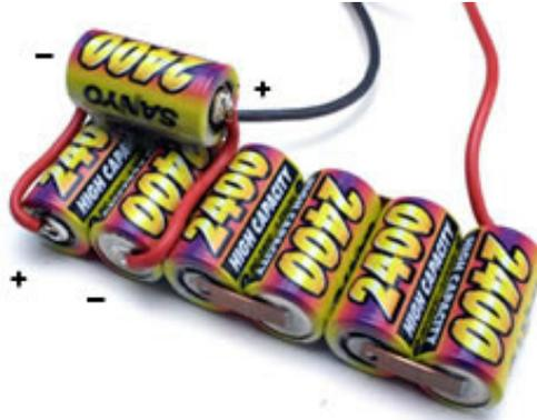
On pack # 2 the cell is mounted on the other side and will need the 2 ½" wires to connect it.
