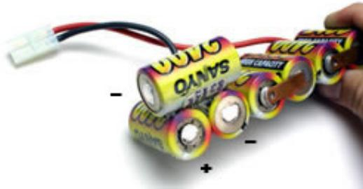
The battery trays in the chassis of the E-Maxx can be used along with the hold downs to make sure that the seventh cell is in the correct position while the glue cures. Allow the glue to set-up overnight before handling the cells. Hang in there. Your pack is almost complete.
