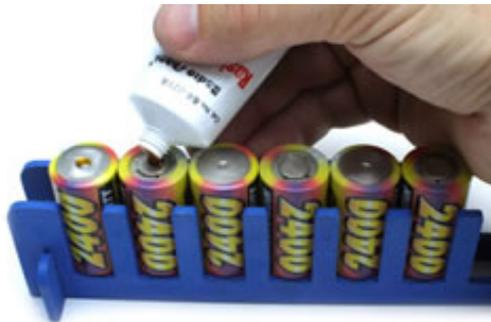
Place a small drop of flux on the end of the cell. Next heat up some solder on the tip of your iron.
