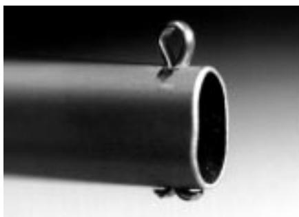
*This is the end of one of Hal Robinson's booms. Hal makes them from aluminum arrow shafts that he heats with a torch until the aluminum begins to change color. He then lets them cool slowly to room temperature before bending curves to match the foot of his sails. After bending, the shaft is flattened between two boards in a vice. Hal says he has to overbend the curve because some of it will come out during the flattening procedure. Note the neat use of a cotter pin as a strap eye.*
