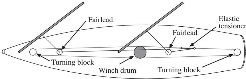
This is the sheeting arrangement used by Jim Linville for his latest US One Meter. The drum winch (a Futaba 5801) drives a loop of 80# Spectra that is lead through turning blocks at the far ends of the hull and held in tension by an elastic stretched between two rings. Sheets are fed to the booms through deck mounted fairleads. The elastic is located so that it can be replaced through the hatch.
