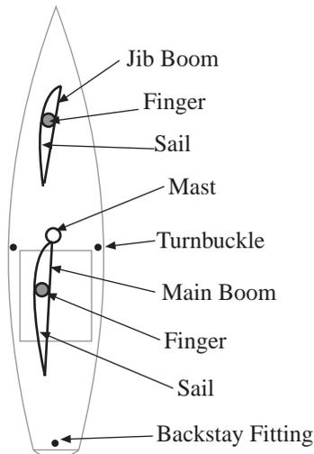
With sails let out set Jib boom approximately 2 deg. beyond right angle. Allow some slack in Main sheet. When sails are pulled in slightly the Jib will be at right
