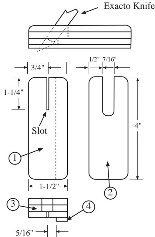
1. 1/4" thick plywood (make one). Notice slot is cut at slight angle.
