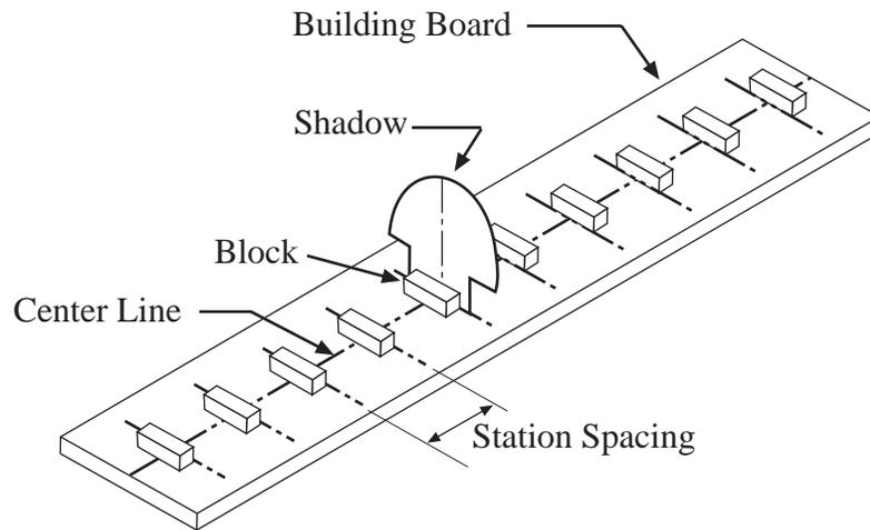
The board has to be “warp-free”. It can be plywood or particle board shelving material. Particle board is a little more difficult to cut and drive nails into than plywood. Size of the board is about 5/8" x 12" x 48". If you want to keep the board clean, cover it with shelf paper.
