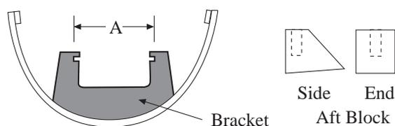
Make the hull bracket from 1/8" plywood. Cut and sand until bracket fits hull and radio board perfectly. Dimension "A" is the width of the radio board. Trim the inside area of the bracket to provide clearance for SCU motor and/or keel mounting bolts and nuts.
