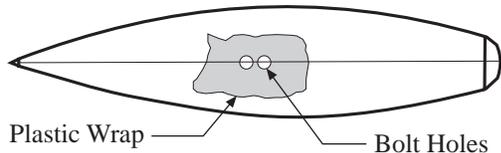
Cover bottom of hull around bolt holes with thin plastic wrap. Tape the wrap to hull. Punch holes in plastic wrap for keel bolts.
