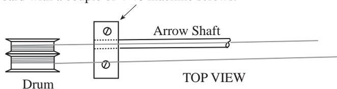
Here's a spiffy way to rig a drum winch for a Soling One Meter or similar yacht. The complete unit slides out of boat with radio board.
