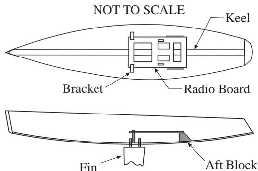
Your equipment dictates the size and placement of the radio board.
