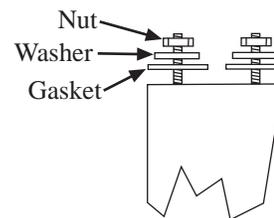
sure to use gaskets, washers and nuts in that order. To prevent water from entering hull through mounting holes. Gaskets can be made from neoprene faucet washers, bicycle inner tube material, etc..
