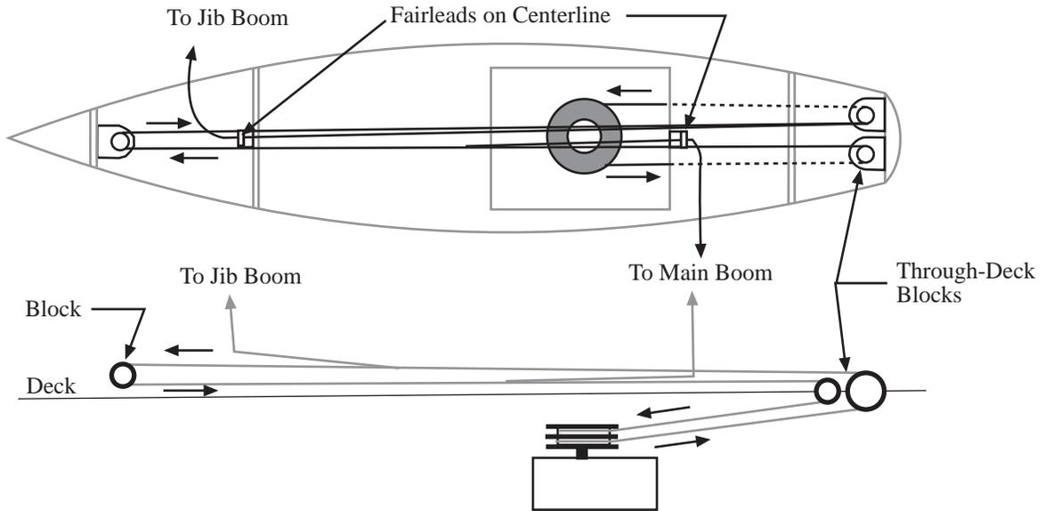
*Note: The side view drawing shows the “Through Deck Blocks” as different sizes, they are not, they are both the same size.*
