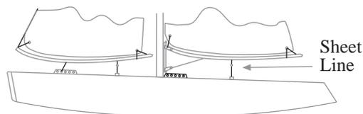
Tape sheets to framework temporarily to get correct sheet length.
