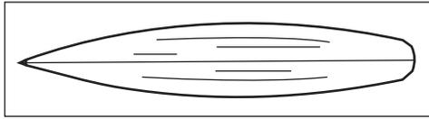
Sand hull smooth with 100 grit sandpaper. Fill in all gaps in planking and any low spots. Finish sand with 120 grit sandpaper.
