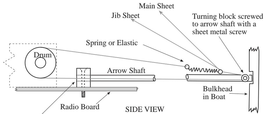
Aluminum Arrow Shaft Block. Drill to fit arrow shaft and mount on removable radio board with a couple of 4-40 machine screws.
