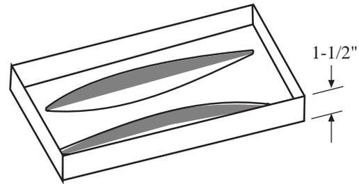
can speed up the process by using your kitchen oven. Three or four hours at 200 degrees F, maybe longer, should do the trick. Let plaster cool. Place plastic wrap (Saran, etc.) over plaster mold. This acts as a parting agent and allows the slugs to be removed from the mold easily.
