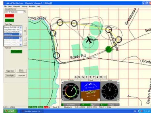
Figure 2. An autopilot controlled UAV flight path between way-points (octagons) plus associated instrument displays.
