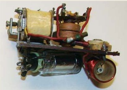
Hitec's new 1/2-ounce 7-channel Optima receiver clearly highlights RC's progress when seen with Bob Aberle's 1953 original Miller hard-tube single-channel 4.5-ounce receiver on the right. We sure have come a long way!
