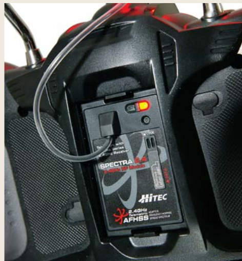
The 2.4GHz AFHSS module mounts in the back of the Aurora just like the modules we have been using for years with 72Mhz systems. You don’t have to give up your 72Mhz legacy gear to enjoy the benefits of the Aurora 9. The 2.4GHz module and antenna can be replaced at will with 72Mhz components.
