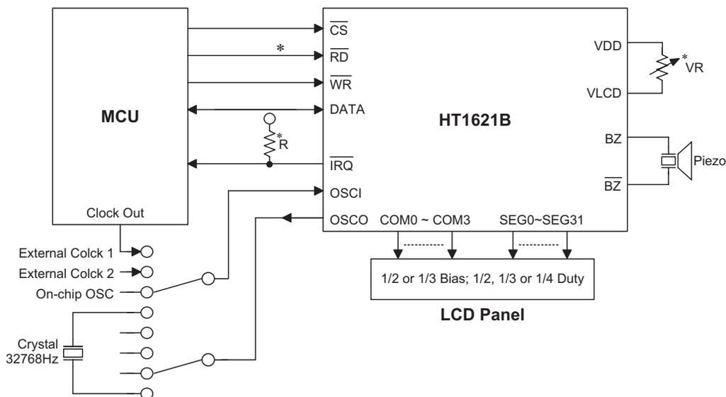
Note: The connection of  $\overline{IRQ}$  and  $\overline{RD}$  pin can be selected depending on the requirement of the MCU.
